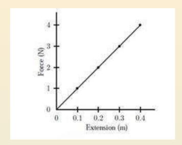
**Hooke's law** is a principle of Physics that states that the force F needed to extend or compress a spring by some distance  $\Delta x$  is proportional to that distance.
